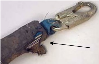
Damaged lanyard shock absorber pouch
